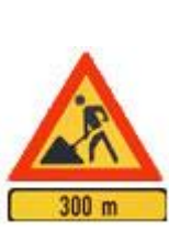
Caution Temporary men at work for specified distance sign
