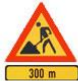
Caution Temporary men at work for specified distance sign
