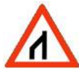
End of dual Roadway left
