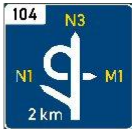
Overhead Pre-advance exit direction
