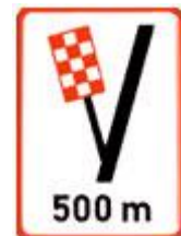
Arrester bed advance exit
